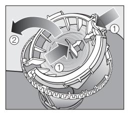
The cover must be opened to clean the inside of the filter:
